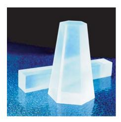
The unique physics capability of crystal calorimetry is the result of its superb energy resolution, hermetic coverage and fine granularity. In high energy and nuclear physics, large arrays of scintillating crystals have been assembled for precision measurements of photons and electrons.
